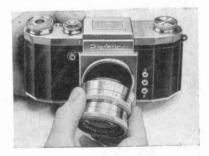
the slightest damage. It is advisable, before exchanging the lenses, to swing the mirror up. Only use a very soft-haired brush to remove any possible uncleanliness from the mirror.
