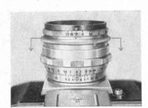
diaphragm number chosen. The milled ring, when springing back into position, will get coupled with the diaphragm ring. For focussing, the diaphragm ring can now be set to the full aperture and, without changing the position of the camera, turned back until it stops at the preset diaphragm number.
